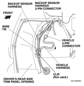
67. Secure the vehicle harness and backup sensor harness to the vehicle harness with one wire tie as shown.
