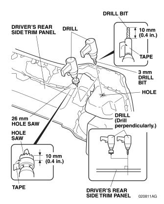
From inside of the driver's rear side trim panel, wear an eye protection and drill one hole with a 3 mm drill bit.
