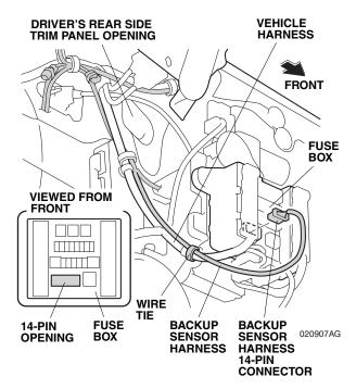
52. Secure the backup sensor harness to the vehicle harness with one wire tie. Go to step 55.
