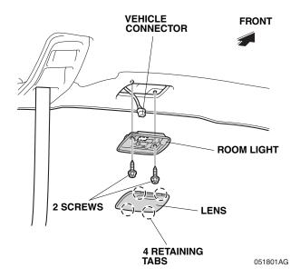
8. Remove the room light (two screws and unplug the vehicle connector).
