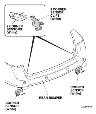
23. Secure two corner sensors (White) with two corner sensor clips (White) as shown.
