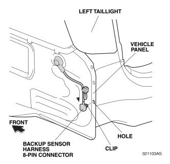
72. Secure the clip on the backup sensor harness to the hole on the vehicle panel as shown.
