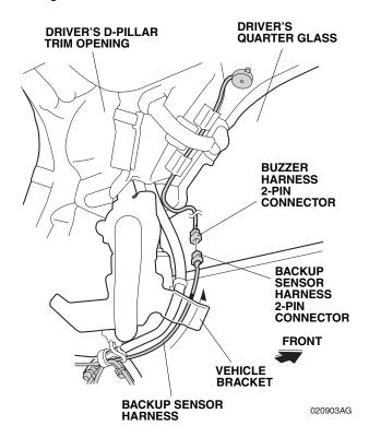
46. Plug the backup sensor harness 2-pin connector to the buzzer harness 2-pin connector.
