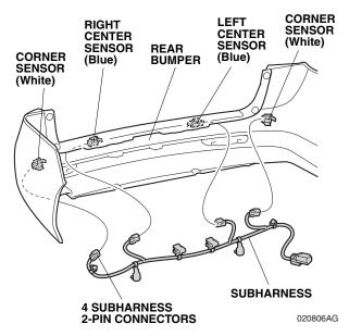
25. Secure two subharness clips to two corner sensor clips (White) as shown.
