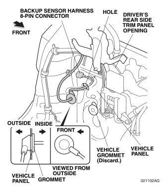
70. Route the backup sensor harness 8-pin connector through the hole, and secure the grommet on the backup sensor harness to the vehicle panel as shown.
