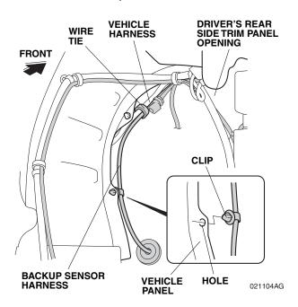
73. Secure the backup sensor harness to the vehicle harness with one wire tie.
