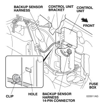
Secure the clip on the backup sensor harness to the hole on the control unit bracket as shown.
